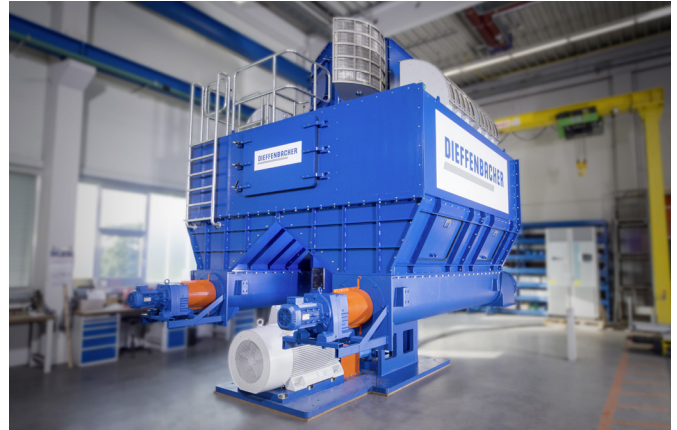
Flameless explosion venting on a grinder machine.
